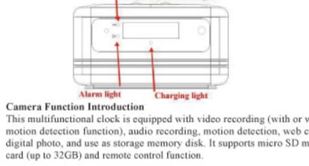
This multifunctional clock is equipped with video recording (with or without motion detection function), audio recording, motion detection, web camera, digital photo, and use as storage memory disk. It supports micro SD memory
